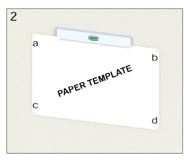
2. In order to facilitate installation we have included a paper template to drill the holes in the wall.
