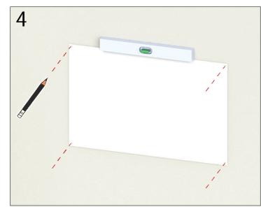
4. Tape the paper template to the wall taking into consideration the position of the mounting holes and the mirror edge. With a level, position the template so that it is perfectly level.
